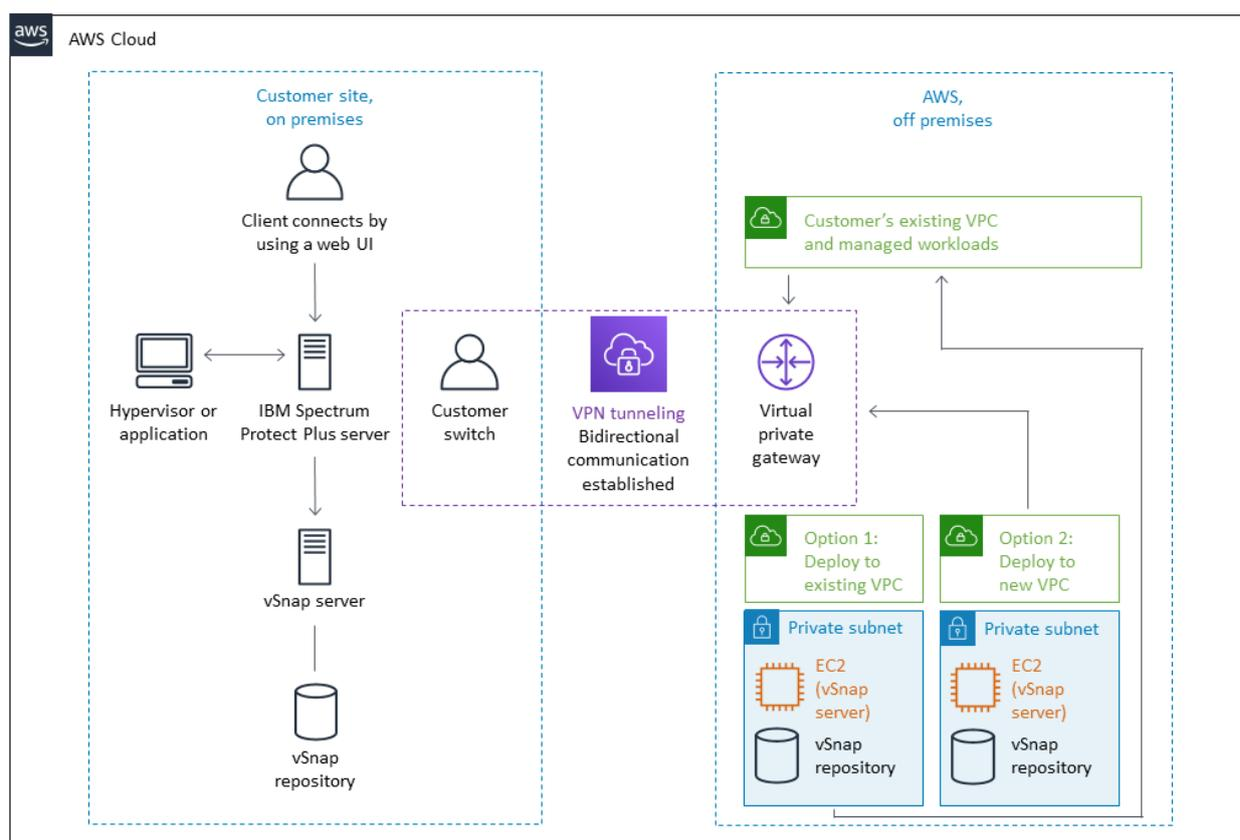
Figure 6: Communication between the vSnap server on AWS and the IBM Spectrum Protect Plus server on premises
