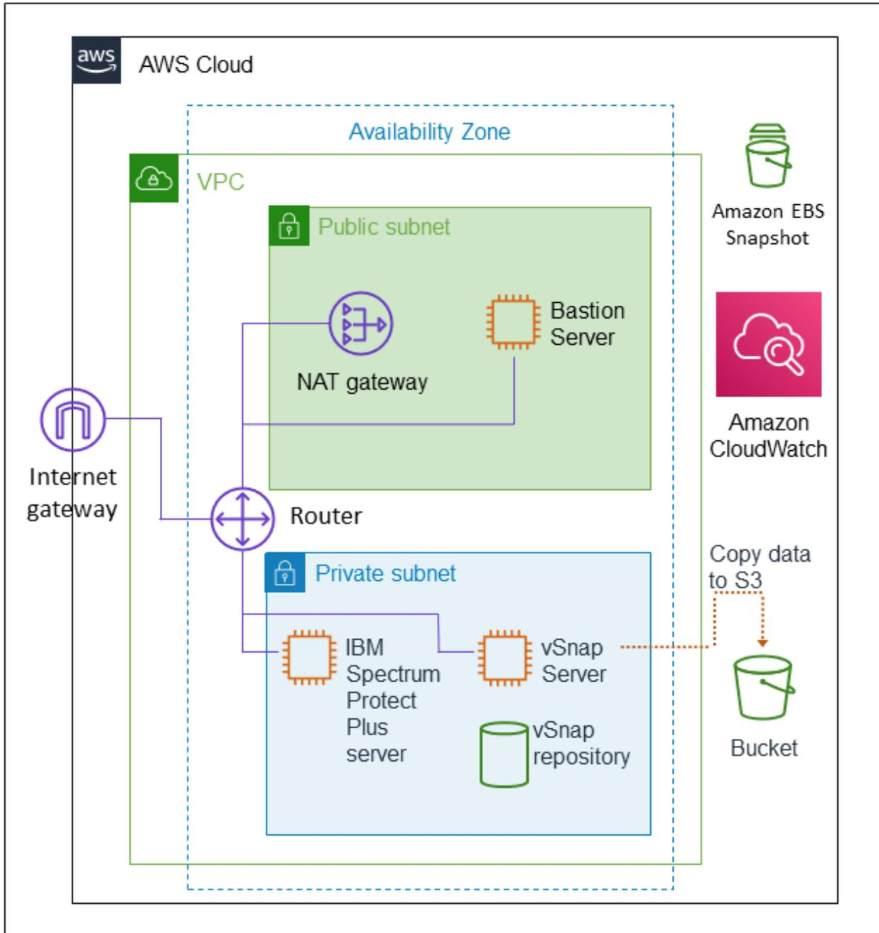
Figure 4: All-on-cloud environment, after deployment to a new VPC
