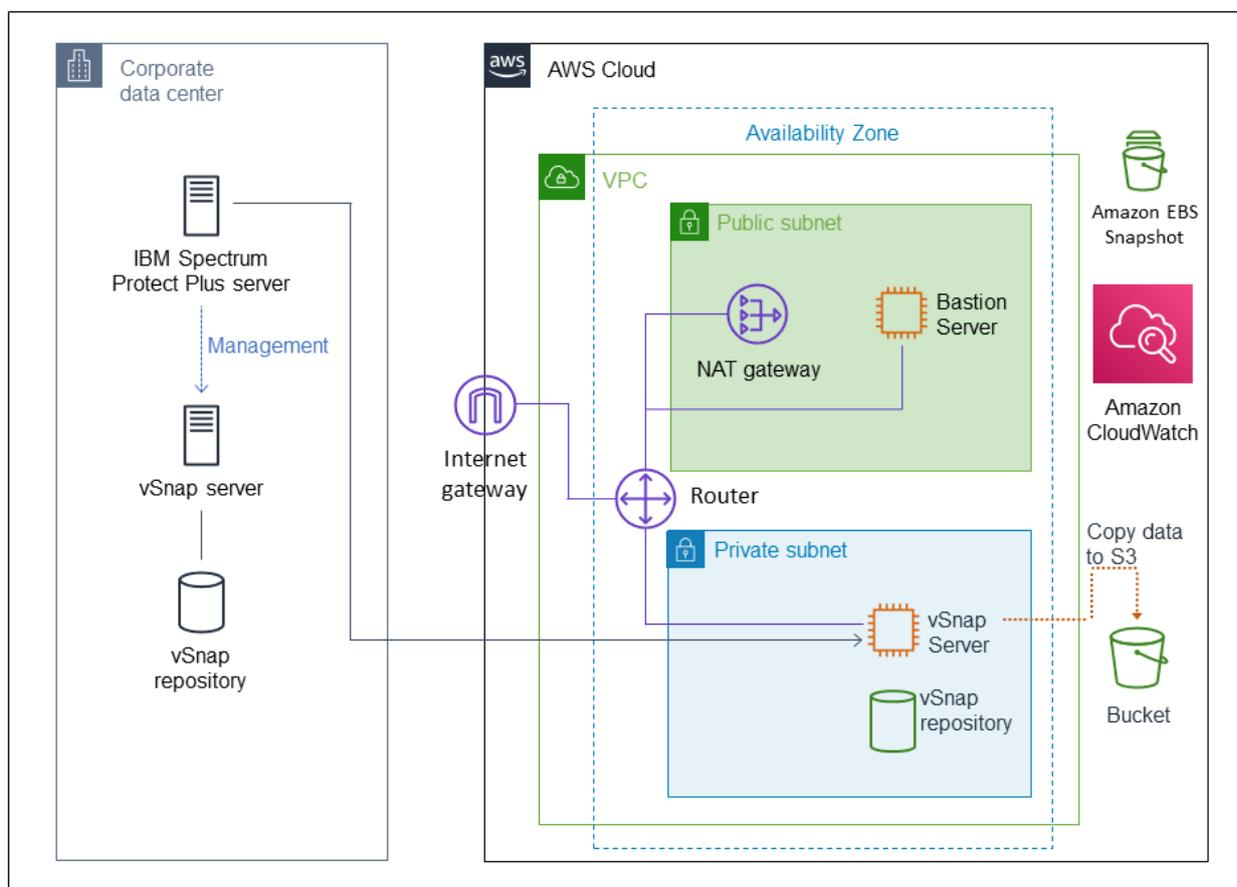
Figure 8: Hybrid environment, after deployment to existing VPC
