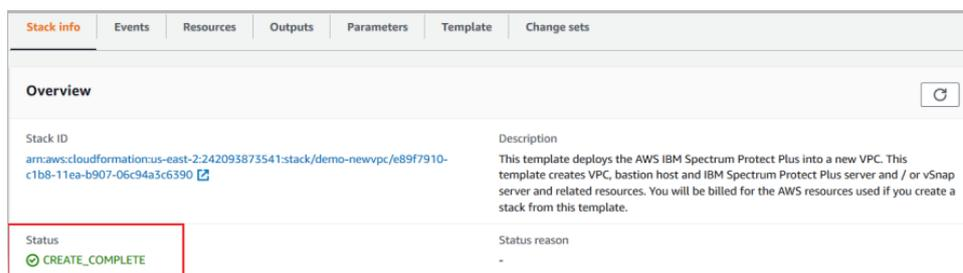
The screenshot shows the 'Stack info' tab in the AWS CloudFormation console. The 'Status' is 'CREATE\_COMPLETE', which is highlighted with a red box. The 'Description' states: 'This template deploys the AWS IBM Spectrum Protect Plus into a new VPC. This template creates VPC, bastion host and IBM Spectrum Protect Plus server and / or vSnap server and related resources. You will be billed for the AWS resources used if you create a stack from this template.'
