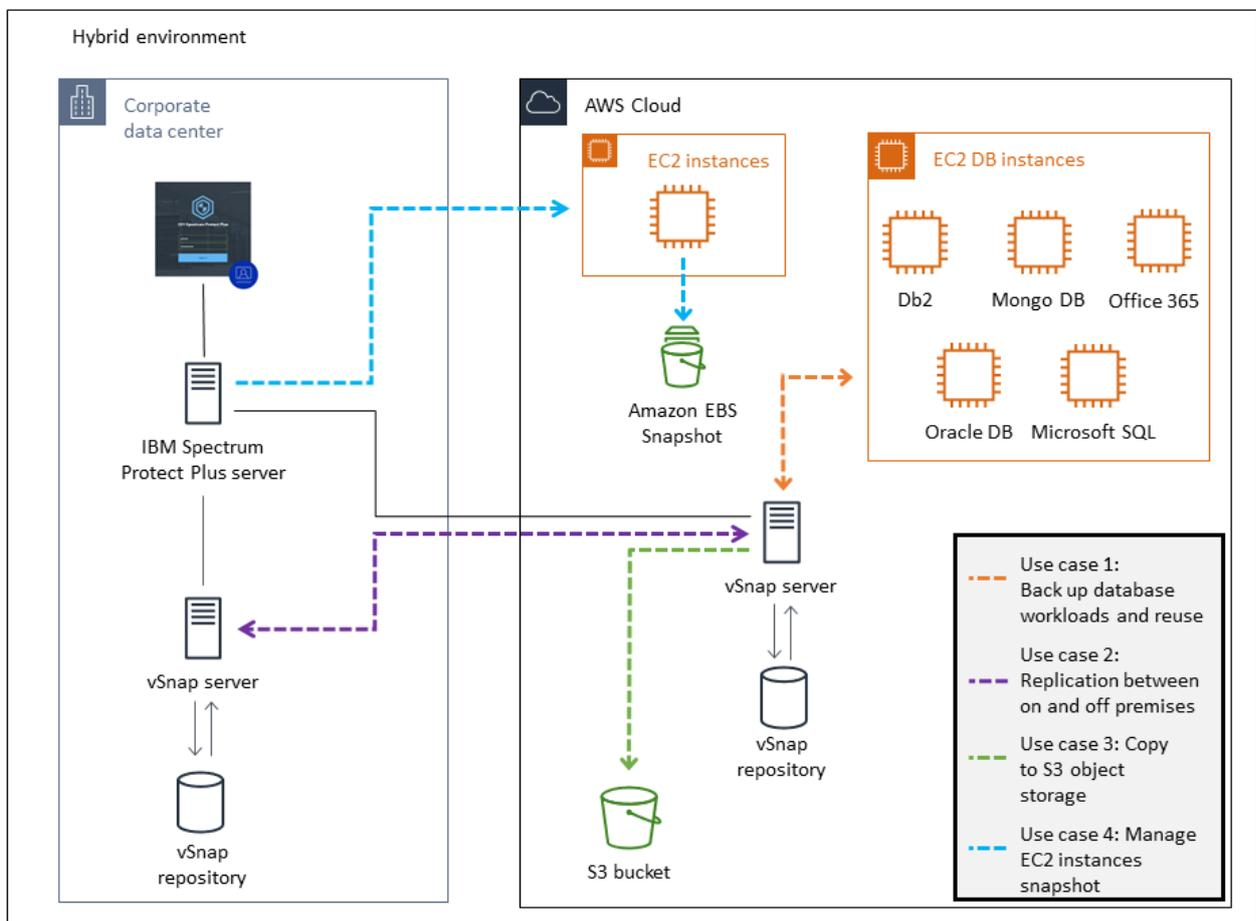
Figure 5: Architecture for a hybrid environment
