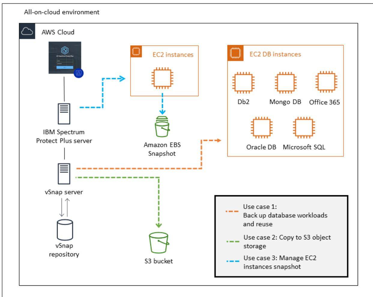
Figure 1: Architecture for an all-on-cloud environment
